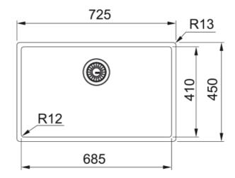
Mythos Masterpeice BXM 210/110-68, Anthracite PVD coating and nanocoating with F-Inox Technology, Stainless Steel, can be installed as a slim-top, flushmount or undermount, 1 bowl without drainer, 680mm x 410mm, 3 1/2". Includes colour coordinated bottom grid and semi-integrated waste with matching overflow. Additional coloured strainer bowl and rollamat can be bought. 50 Year Guarantee on all Franke sinks. 50 Year Guarantee on all Franke sinks.
