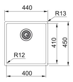
Mythos Masterpeice BXM 210/110-40, Anthracite PVD coating and nanocoating with F-Inox Technology, Stainless Steel, can be installed as a slim-top, flushmount or undermount, 1 bowl without drainer, 400mm x 410mm, 3 1/2". Includes colour coordinated bottom grid and semi-integrated waste with matching overflow. Additional coloured strainer bowl and rollamat can be bought. 50 Year Guarantee on all Franke sinks.
