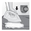
2 Press and release the steam boost button for a powerful boost of steam to remove stubborn creases.
